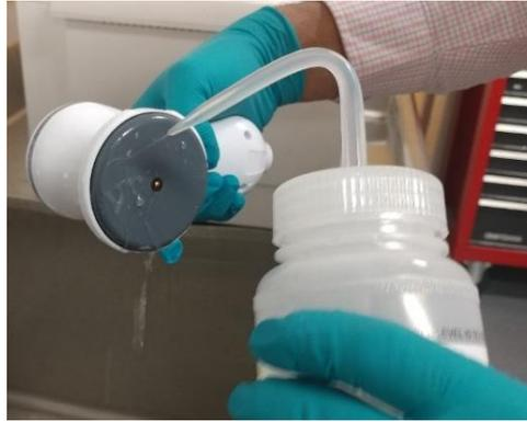
After rinsing the surface, place tip of bottle against the gap and rinse thoroughly around the entire circumference between the electrode and the housing. Do not hold handpiece under running water. Only rinse client contacting surfaces.
